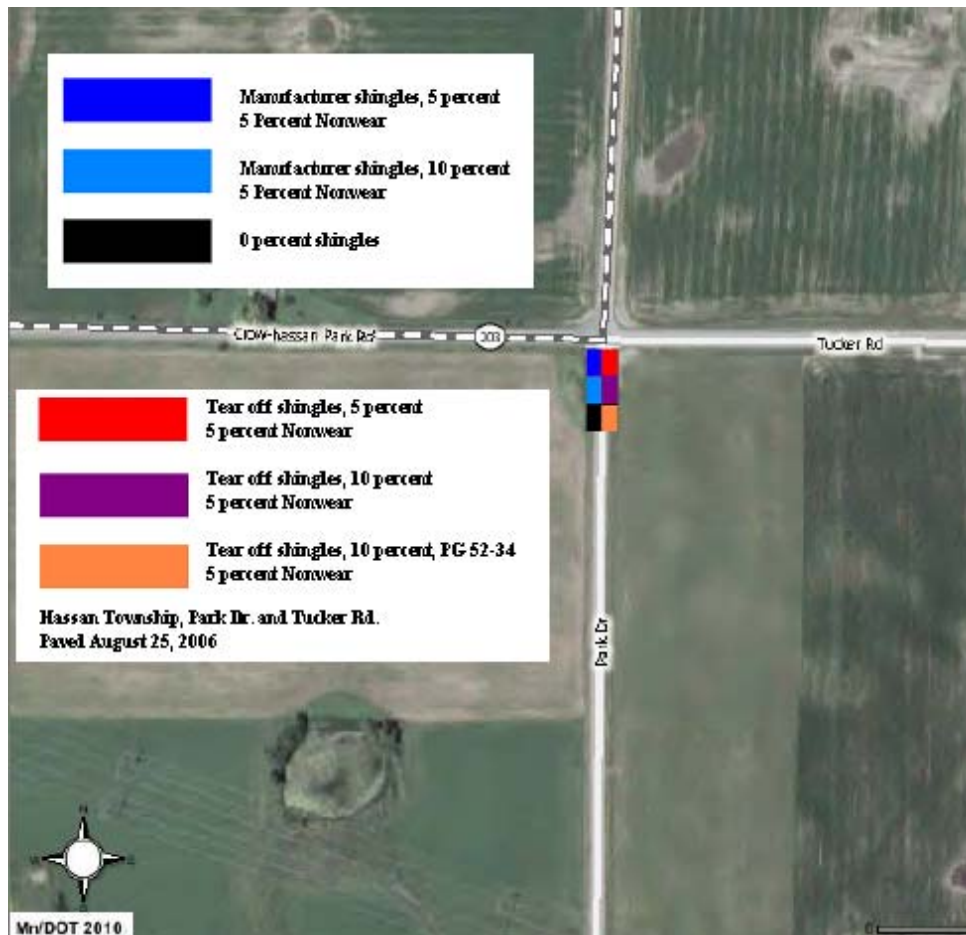
Figure 5.5. Test Section Location in Hassan Township
